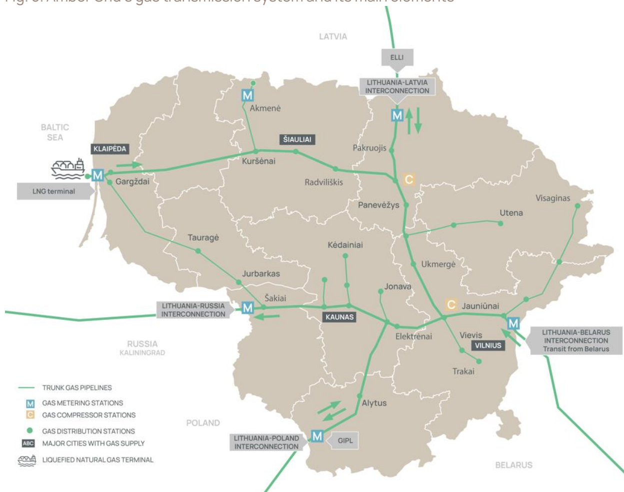
Fig. 5. Amber Grid’s gas transmission system and its main elements
